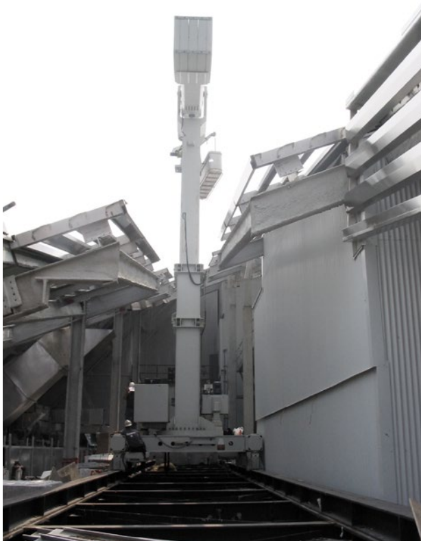
Hydraulically operated telescopic slewing mast
