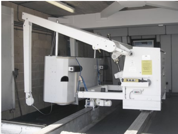
► Retractable jib arms for garage/parked position
