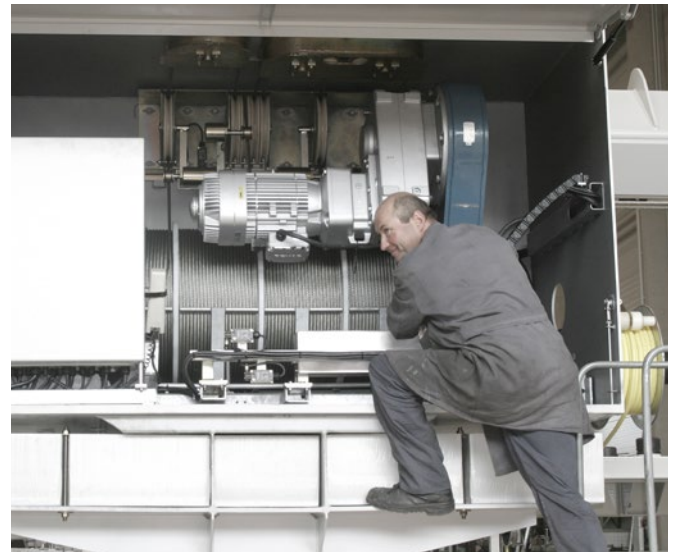
► High-performance hoist unit, approx. 4,000kg lifting capacity.
